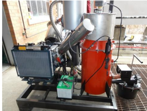
Engine Exhaust Pyrolyzes Chips
