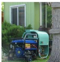
Ngen Eco5 5 kW Pellet Gasifier, Colorado www.ngenpower.com
