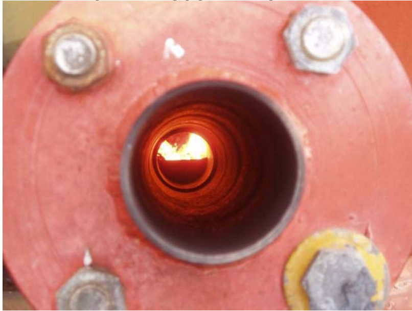
WOOD CUBES IN COMBUSTION ZONE OF GASIFIER AS SEEN THROUGH AIR NOZZLE
