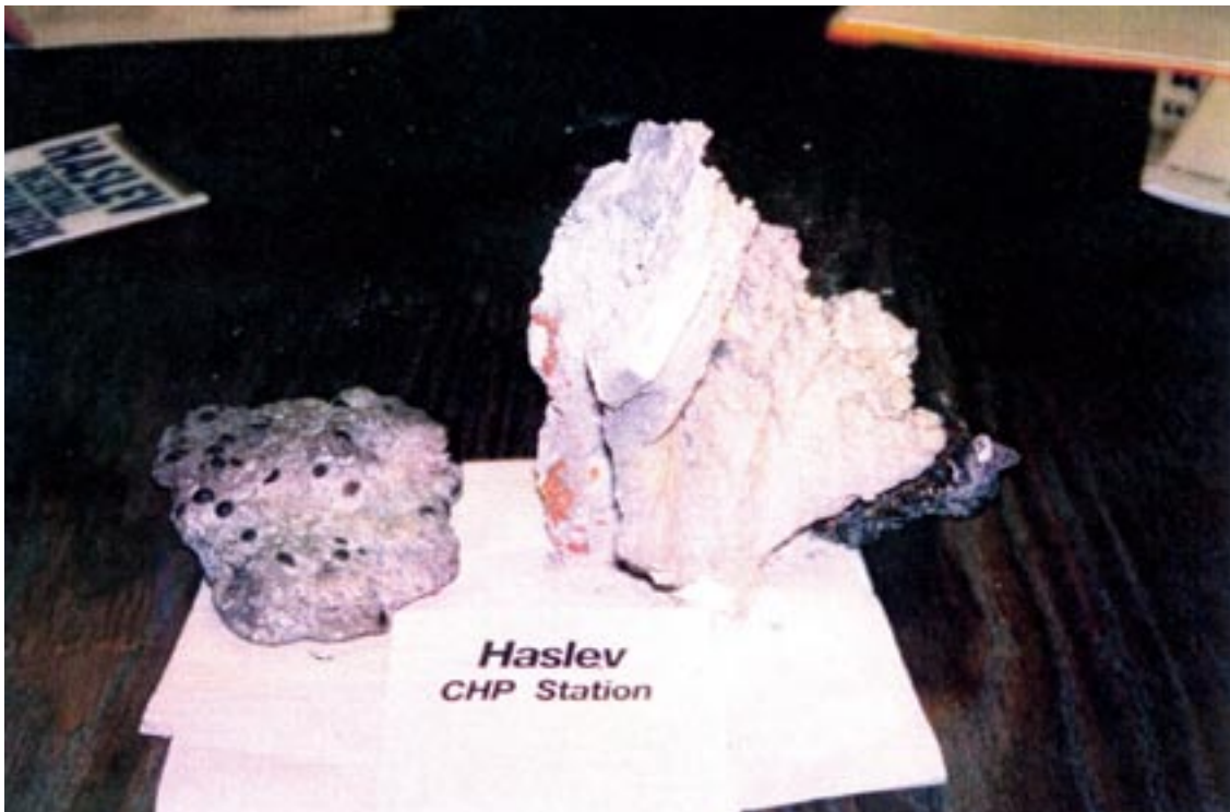
Figure 10 Superheater Deposits from Straw Fired Stoker Grate-2 (Haslev, 1993)
