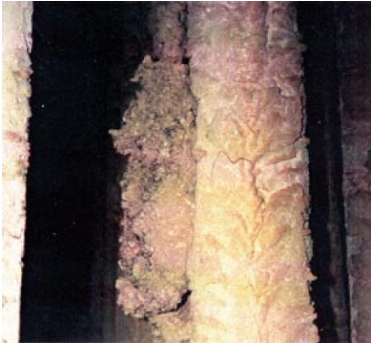
Figure 32 Superheater deposits from Wood-Straw Blend, Grate-1
